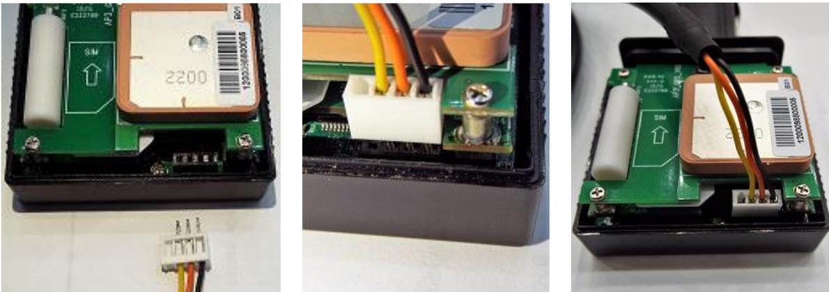
Note that the black wire (GND) is on the side of GPS patch-type antenna, and yellow wire is on the side of polar-type antenna. Once it is done, please open a terminal emulator with serial port as noted before with setting of 57600-N-8-1 and line characters of "\r\n" (or 0x0D 0x0A).
