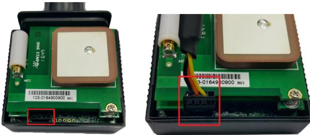
Note that the black wire (GND) is on the side of polar-type antenna, and yellow wire is on the side of GPS patch-type antenna. Once it is done, please open a terminal emulator with serial port as noted before with setting of 57600-N-8-1 and line characters of "\r\n" (or 0x0D 0x0A).
